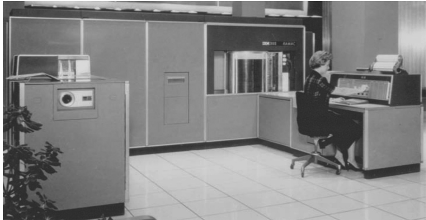
FIGURE 5.17.6 The RAMAC disk drive from IBM, made in 1956, was the first disk drive with a moving head and the first with multiple platters. The IBM storage technology Web site has a discussion of IBM's major contributions to storage technology.
