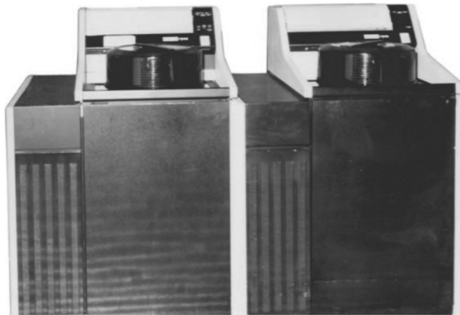
FIGURE 5.17.7 This is a DEC disk drive and the removable pack. These disks became popular starting in the mid-1960s and dominated disk technology until Winchester drives in the late 1970s. This drive was made in the mid-1970s; each disk pack in this drive could hold 80 MB.
